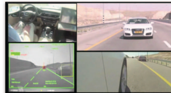
Mobileye's single-camera system can respond to traffic lights and negotiate intersections
